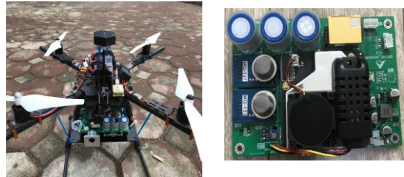
Figure 4: UAV with sensor board to collect data
