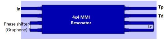
Figure 2. Microring resonator based on only one multimode waveguide structure
