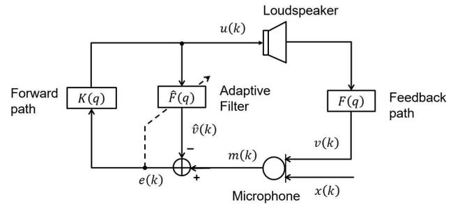
Hình 1. The diagram of a hearing aid using standard AFC.
