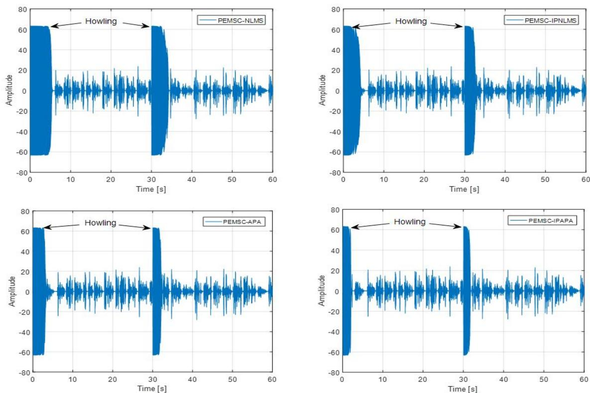
Hình 7. The output signal of the PEMSC-IPAPA and baselines, with a sudden change of feedback paths from  $F_1$  to  $F_2$  after 30 s, concatenated speech as incoming signal.
