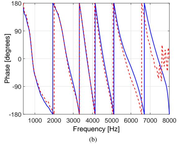
Hình 4. Measured feedback paths: a) Amplitude responses, b) Phase.
