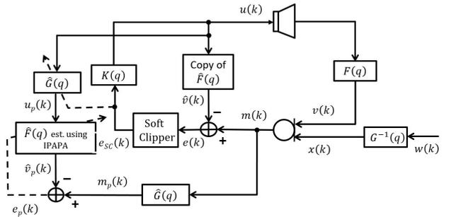
Hình 3. Block diagram of the proposed PEMSC-IPAPA approach.
