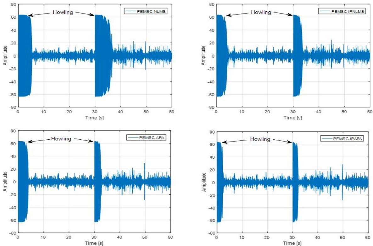
Hình 8. The output signal of the PEMSC-IPAPA and baselines, with a sudden change of feedback paths from  $F_1$  to  $F_2$  after 30 s, music as the incoming signal.
