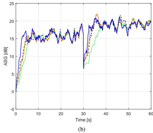
Hình 6. Performance of the proposed methods with music input, feedback path changes from free-field ( $F_1$ ) to telephone-near ( $F_2$ ) after 30 s, a) MIS, b) ASG.
