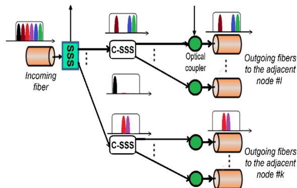
Fig. 2. Two-stage coarse granular routing principle.
