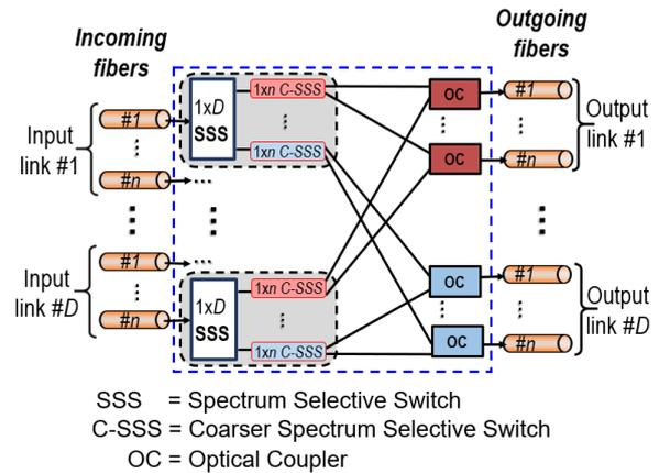
Fig. 1. Developed coarse granular routing elastic optical cross-connect architecture.
