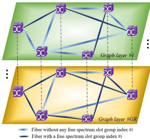
Fig. 3. Auxiliary multi-layer light-path graph of the network.
