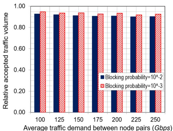
Fig. 8. Accepted traffic volume comparison with different connection blocking probability.
