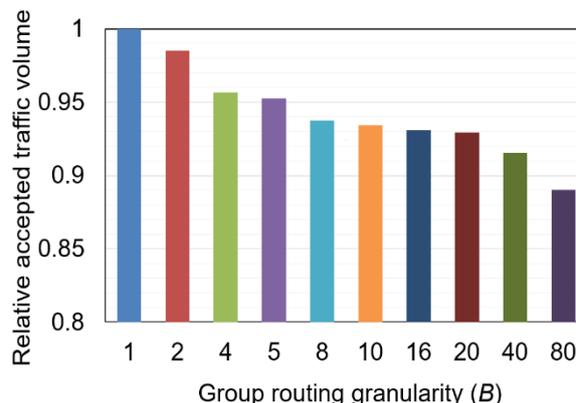
Fig. 9. Dependence of the accepted traffic volume on the group routing granularity.
