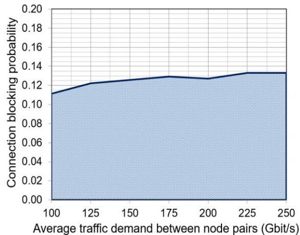
Fig. 6. Connection blocking probability versus average traffic demands between node pairs.
