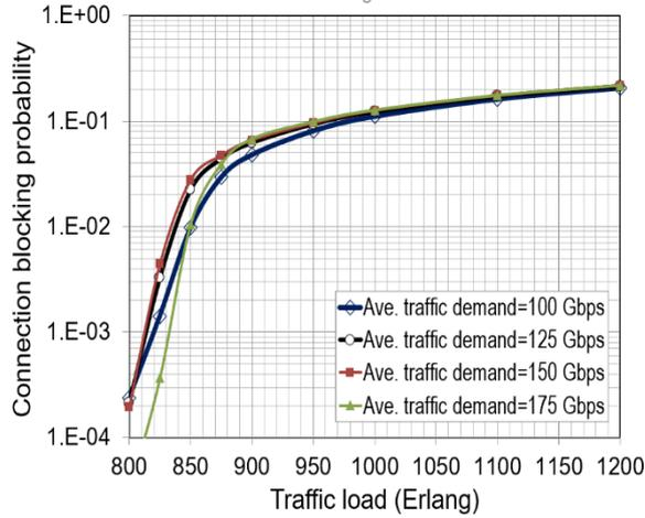
Fig. 5. Connection blocking probability versus traffic load with different values of the average traffic demands requested.
