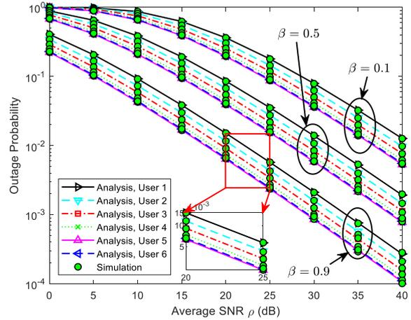
**Figure 5: The OP at each user with  $M = 6$  versus average SNRs.**
