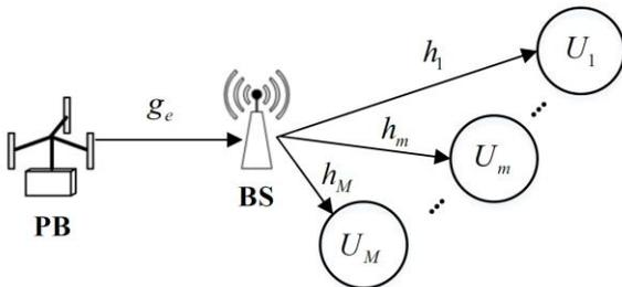
Figure 1: System model of downlink NOMA energy harvesting for multiple users.
