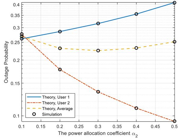
Figure 2: User OP versus power allocation coefficient.
