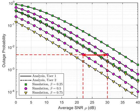
**Figure 3: The OP as a function of the average SNR with the influence of the time allocation coefficient for  $M = 2$ .**
