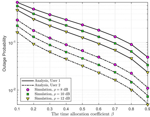
**Figure 4: The OP of each user versus the time allocation coefficient with  $M = 2$  users.**
