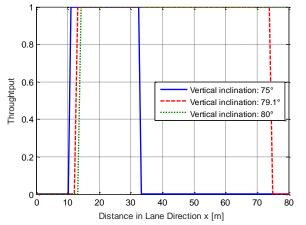
Fig 6. Throughput in 1st lane with different vertical inclinations.
