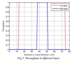
The system throughput is investigate versus the distance in lane direction x in Fig. 5. The figure shows that the system throughput reaches the maximum value of 1 Mbps when the vehicles are at the communication area. This is due to the fact that the system provides error-free in communication.
