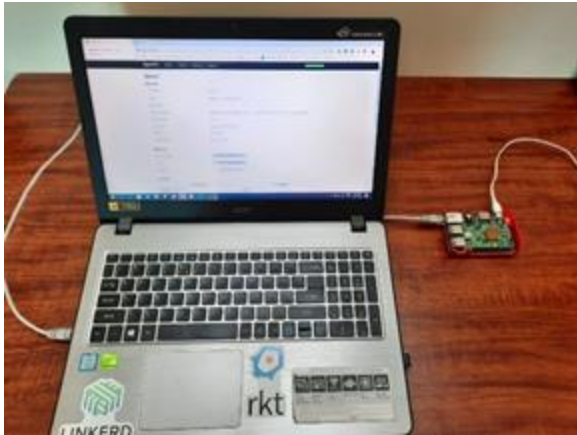
Figure 2. The developed SDN-based Wi-Fi AP prototype and Web-based GUI.
