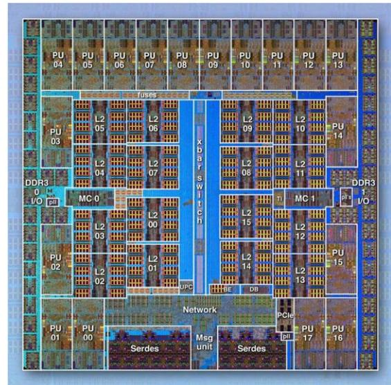
Fig.3. Blue Gene Q Compute Chip - IBM’s Blue Gene Q compute chip contains 18 cores and dual DDR3 memory controllers for 42.7 GB/s peak memory bandwidth.
