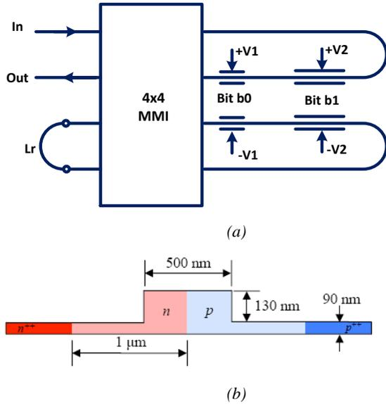
Fig 4. (a) Scheme of a PAM-4 signaling based on a 4x4 MMI coupler and (b) PN junction phase shifter with reserve bias and the structural parameters of the waveguide
