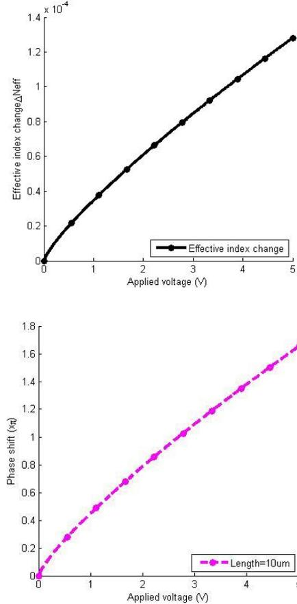
Fig. 9 Effective index change and phase shift with the electrode length of 10um
