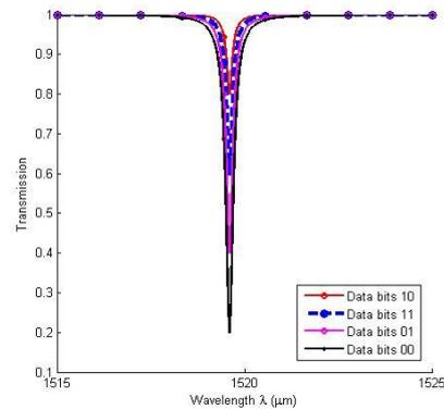
Fig. 10 Transmission of the proposed structure for input data bits 00, 01, 10, 11
