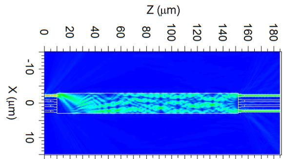
Fig. 6 Power transmissions through the 4x4 MMI at the optimized length 141.7  $\mu\text{m}$ , input signal is at port 1
