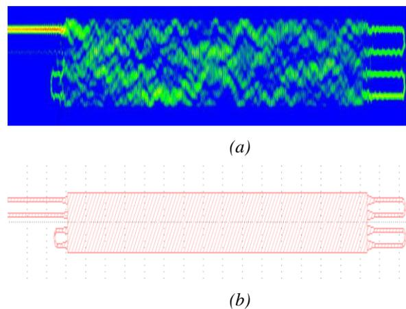
Fig. 7 FDTD simulation of the whole device when input signal is at port 1
