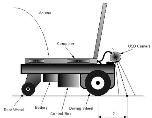
Figure 13. The model of the mobile robot
