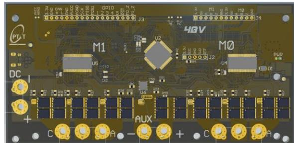
Figure 12. BLDC motor driver
