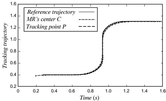
Fig. 9 WMR's movement tracking reference path
