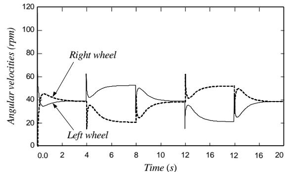
Figure 5. Angular velocities of two wheels
