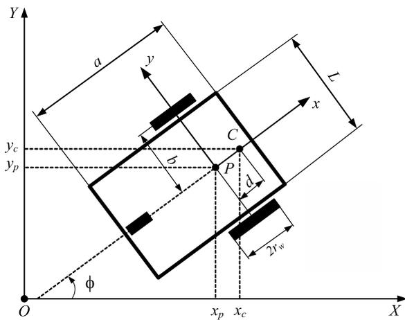
Figure 1. Mobile platform configuration
