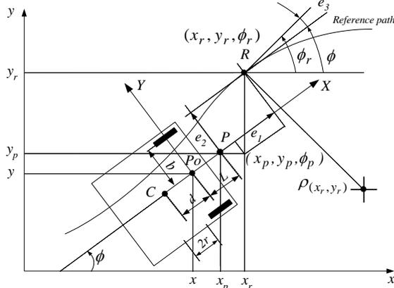
Figure 2. Scheme for deriving WMR kinematics equations
