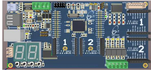
Figure 11. Motion controller is based on STM32
