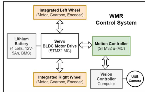
Figure 10. The configuration of the control system
