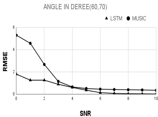
Figure 9. Compare RMSE (degrees) of DOA algorithm based on LSTM and MUSIC methods with different SNR values
